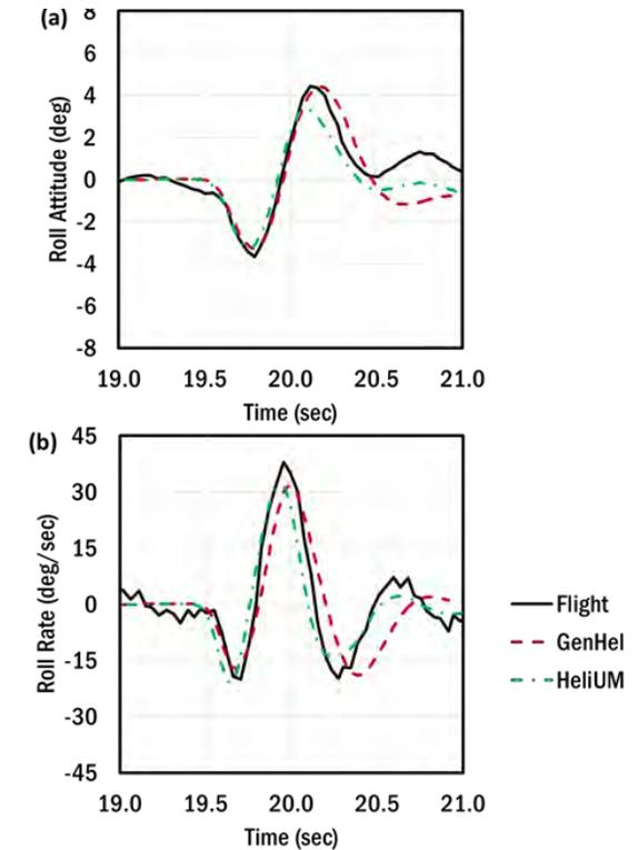
**Figure 25: Body Dynamic Response to Roll Doublet at 200 knots**
