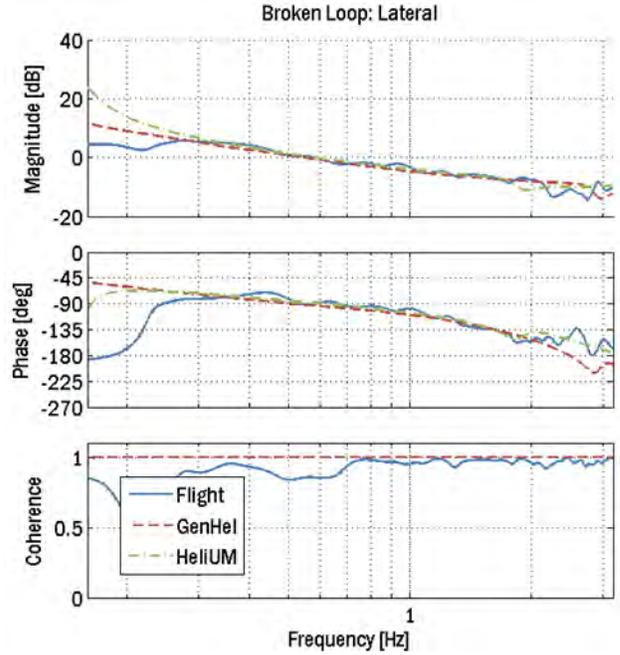
Figure 18: Lateral Broken-Loop Response
