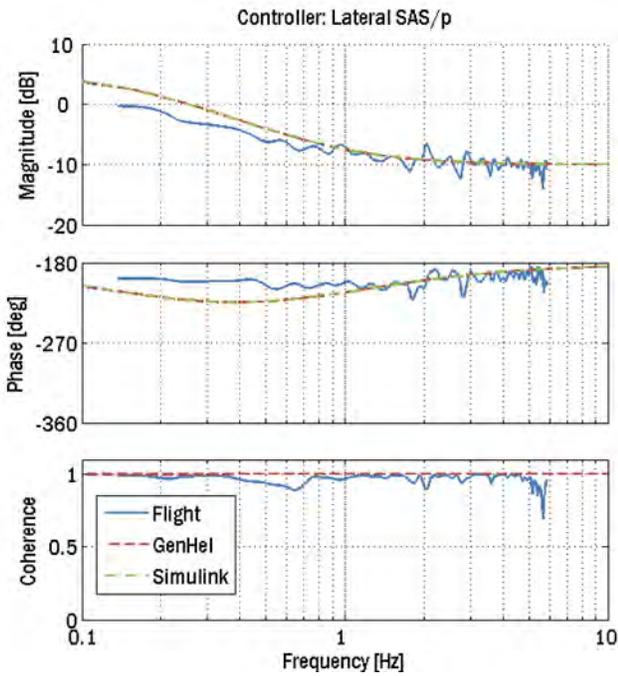
Figure 16: Lateral Control System Response to Roll Rate
