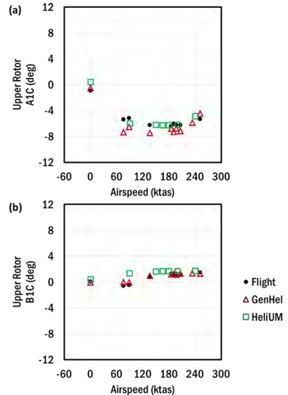
**Figure 4: Upper Rotor Trim Cyclic Pitch (a) Longitudinal Cyclic Pitch vs. Airspeed (b) Lateral Cyclic Pitch vs. Airspeed**
