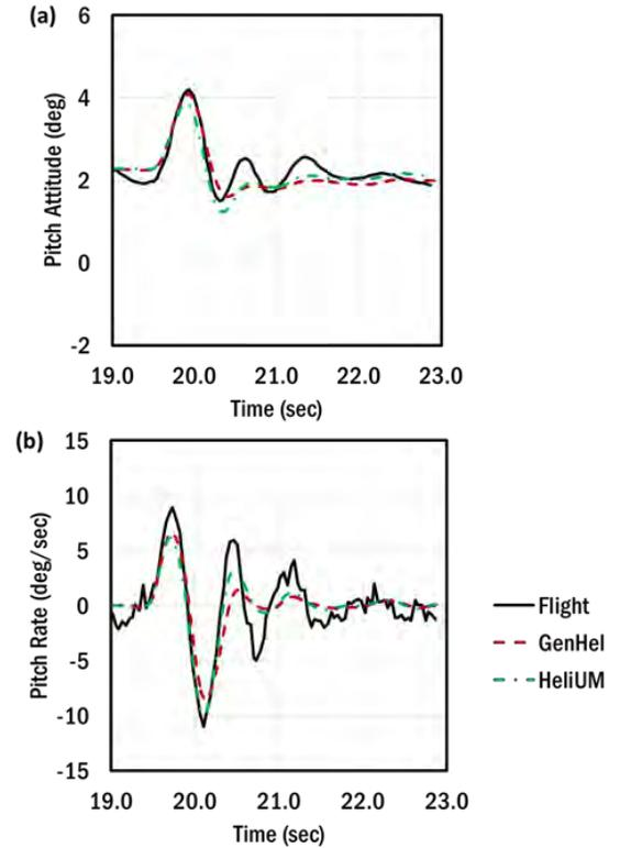
**Figure 24: Body Dynamic Response to Pitch Doublet at 200 knots**
