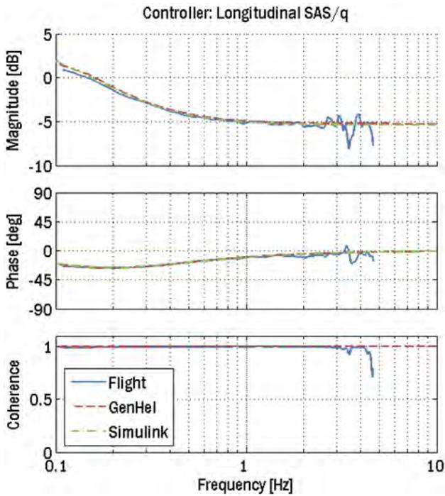
Figure 17: Longitudinal Control System Response to Pitch Rate
