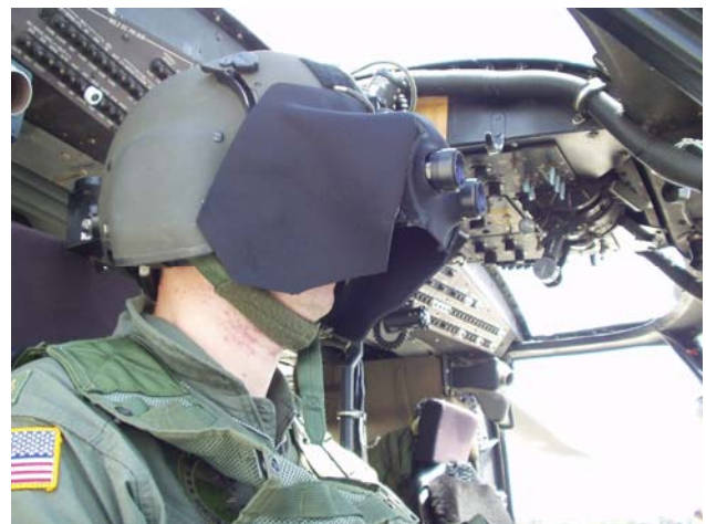
Figure 30. Modified Night Vision Goggles for Simulation of Degraded Visual Environment (UCE 2)
